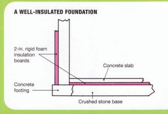
colder areas. Without any insulating barrier to slow it down, some of the heat in your house is absorbed by the concrete walls and floor of your basement. This makes the foundation heat sink—a kind of negative radiator.
